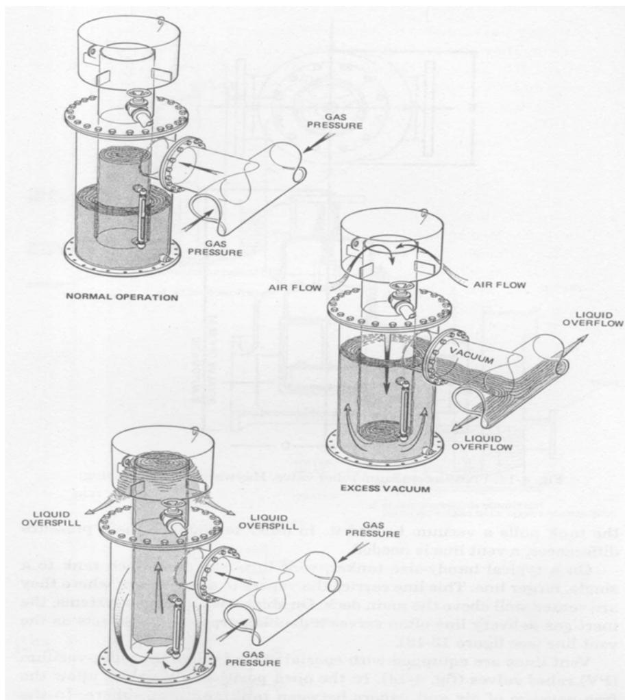
**Figure 2.5 – The design and operation of a P/V breaker<sup>3</sup>**
