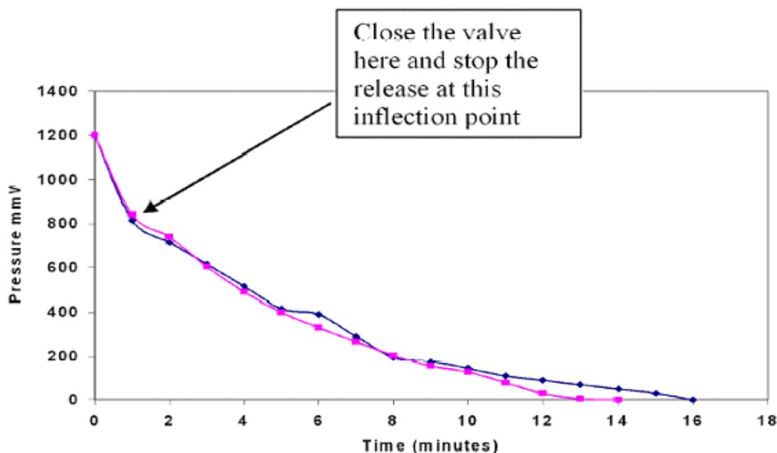
**Figure 4.2 – A mast riser release**
